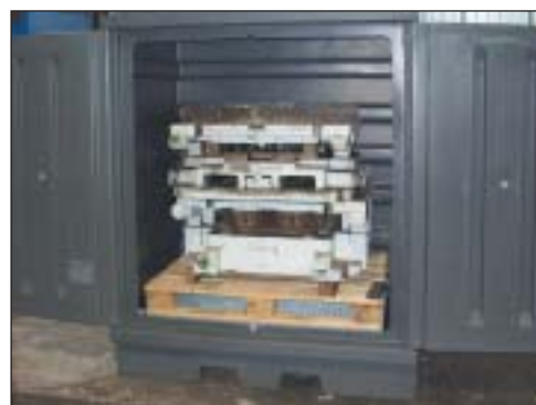
PE-200-EP8 under a test load of 2400 kg
